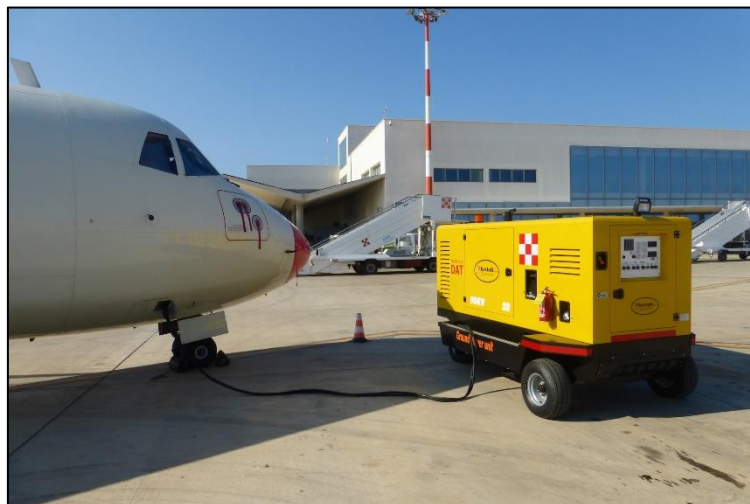
Figure 3 : unité mobile GPU (source : Airport Suppliers)
